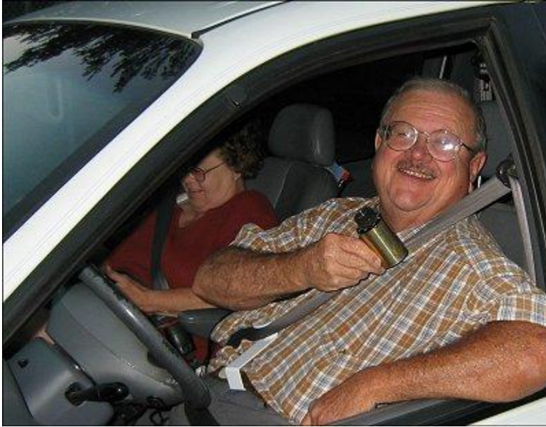
Photo 6: Dick, NOØT, and Kay, WA5DYC used signal strength to find the fox. Dick is holding a variable RF "step attenuator" which is the gold cylinder with the black knob atop. This device weakens signals passing through it, which is handy when closing in on the fox.
