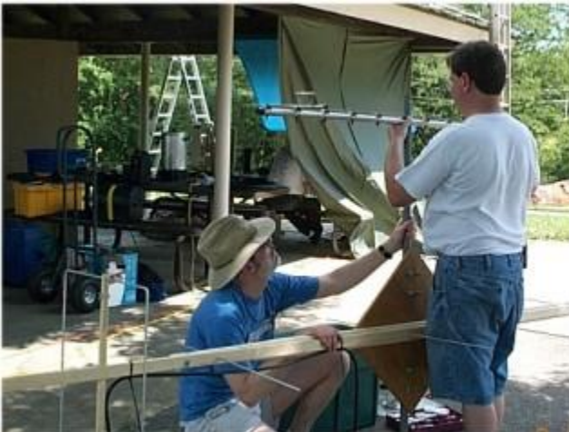
Photo 9: KYØDR, David, is constructing a 2-meter Quagi antenna (A Quagi antenna has reflector and director elements like a Yagi, but is driven by a loop like a Quad.)
