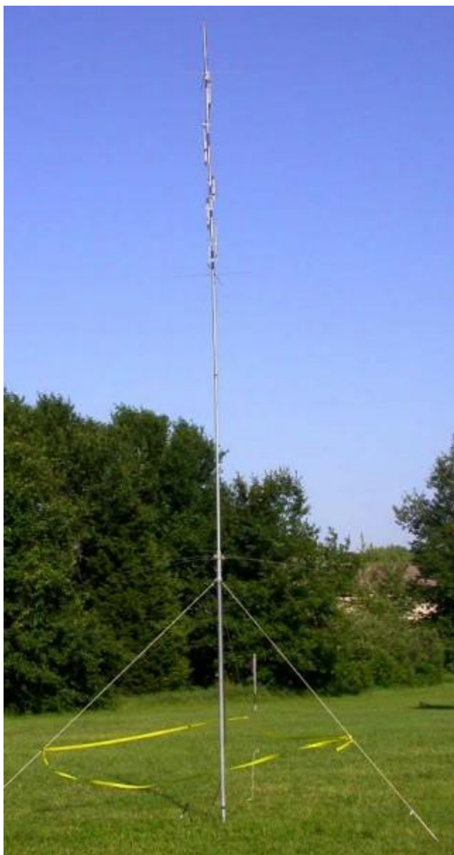
Photo 4: Stan (KD0G) provided the vertical trap multiband antenna for the CW station. We also used a wire (not visible in this photo) for the SSB station. According to Bill (KA2FNK), we experienced significant interference between the two HF stations this year, and better grounding is in order for next year!
