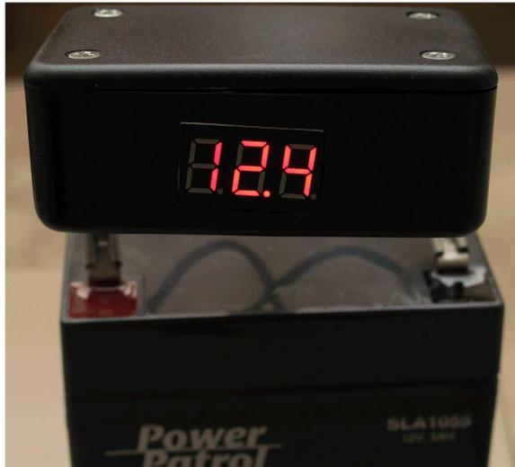
*Figure 1: The EZ-Volt Meter Measuring a 12 Volt SLA Battery*
