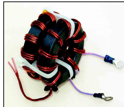
Figure 6—Impedance transformation is accomplished with a 1:1 balun and a 1:2.25 unun, each wound on a separate ferrite core and held together with cable ties. In this photo, the 1:1 balun (with bifilar winding) is toward the front. See text and Figure 5 for details.
